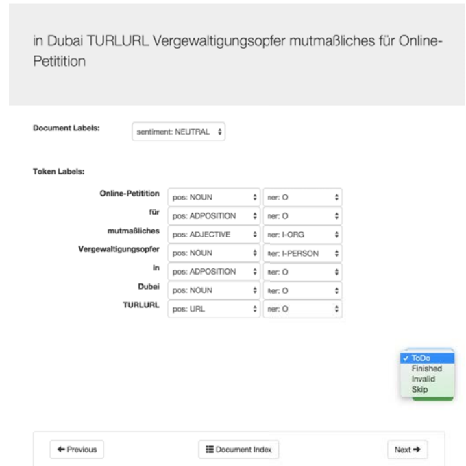
Figure 1: Screenshot of the annotation tool interface. The text of a tweet is at the top followed by the sentiment label dropdown menu. Below there is a column with the tokens and rows for each annotation (PoS and NER). Annotators manually fix the errors inherent in the automatic pre-tagging step previously described. Finally, a dropdown menu allows marking the annotation of the document as "To Do", "Finished", "Invalid", or "Skip". Note that in this example, the labels have not yet been manually corrected.
